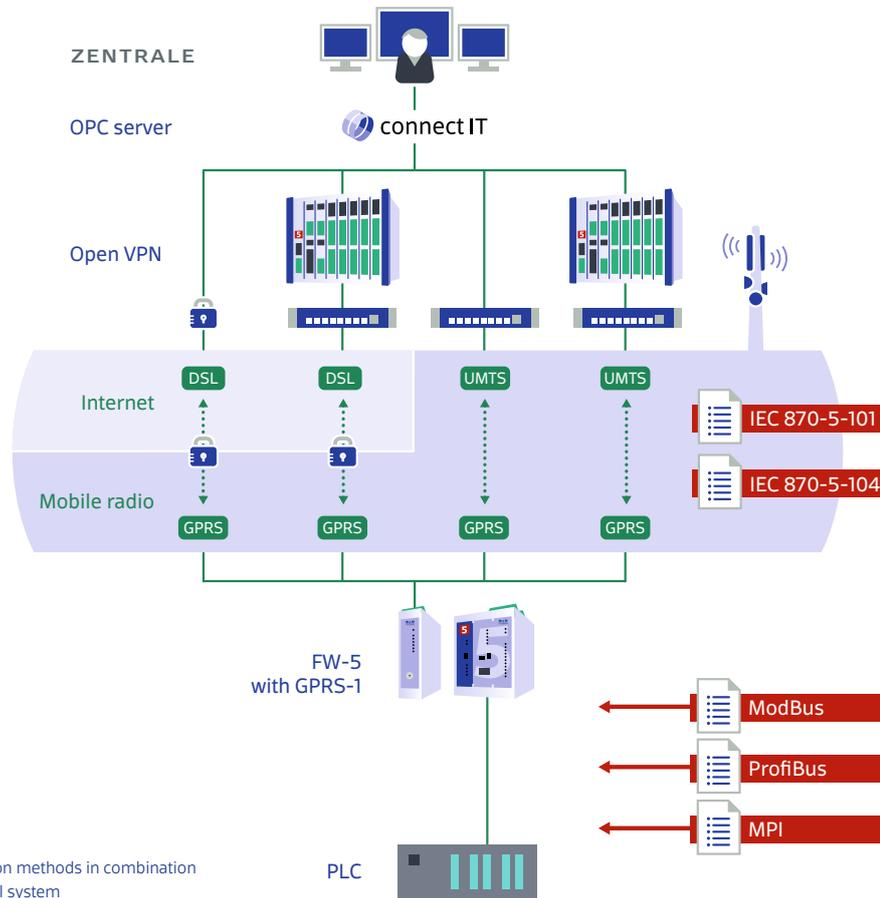
Recommended connection methods in combination with the FlowChief control system
